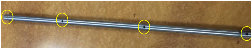
Tube 1b (4 holes in line with each other with a taper at the end)
