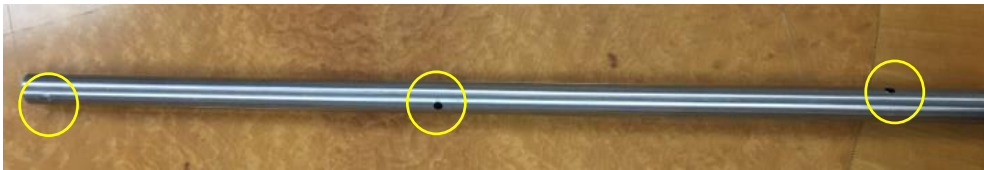
Tube 1a (3 holes with two on a 90 degree angle to the 3 rd )
