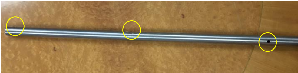
Tube 1b (4 holes in line with each other with a taper at the end)
